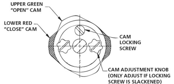
Figure 3. Top view of the cam shaft assembly.
